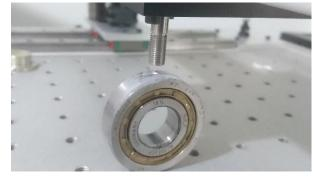
point is clearly indicated by the incident light from the reflection probe with 200um core diameter.
