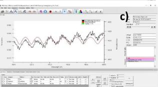
**Figure 1**: Screenshots from the fitting of the specular reflectance spectra. The theickness of the grease depends strongly on the measuremnt point due to the way of application (spraying by hand)
